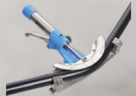
↑ PIPES IN THE DIMENSIONS OF D16 AND D20 CAN BE BENT EFFORTLESSLY BY HAND AND USING A BENDING MACHINE UP TO D50.
