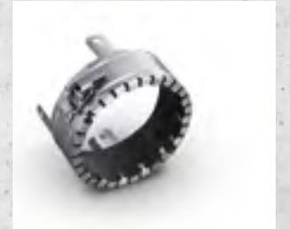
**The Geberit fire protection sleeve RS90 Plus** prevents fire from spreading via the drainage system. Under the influence of heat, the material in the fire protection sleeve swells, completely compressing the discharge pipe and thereby preventing the fire from spreading to other floors or rooms.
